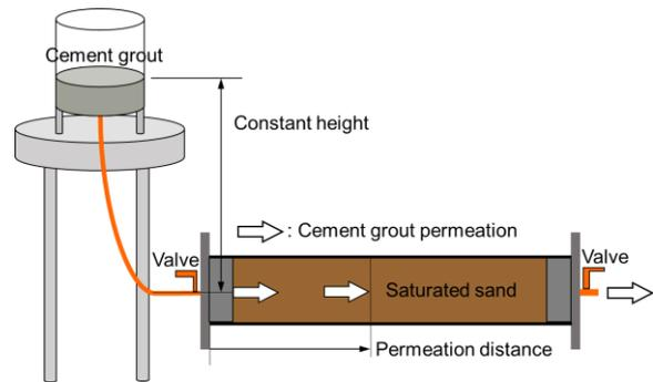
Figure 6. Column permeation test for saturated sand.
