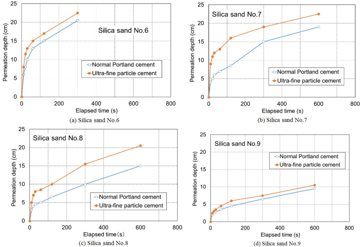
Figure 8. Cement grout permeation test results into dry sands
