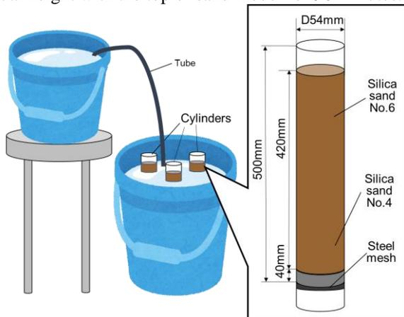
Figure 4. Saturation method of sand model.
