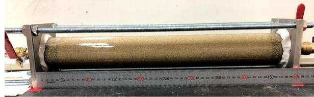
Figure 5. Column with saturated sand.
