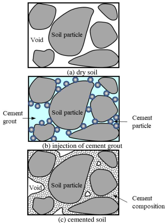
Figure 1. Cement grouting into sandy soil.
