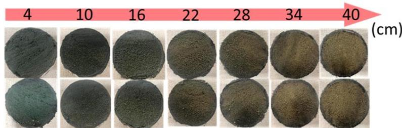
Figure 11. Cement grout permeation test results into saturated sand.
