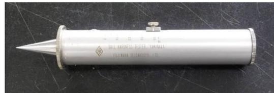
Figure 7. Portable soil hardness tester.
