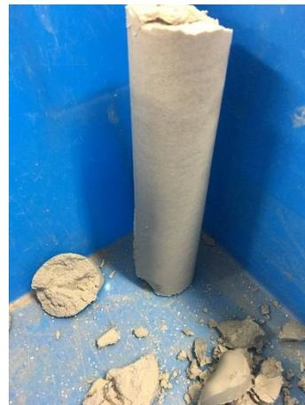
Figure 9. Cemented sand mass after column permeation test.
