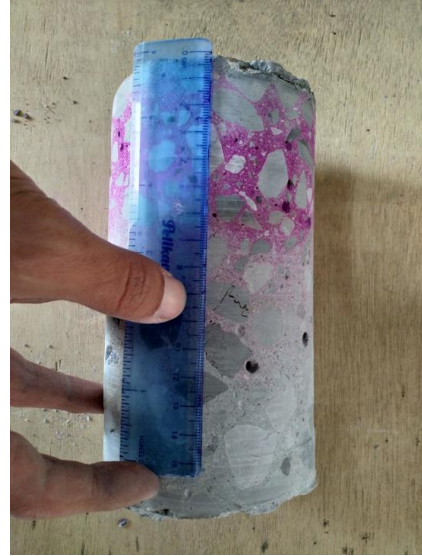
Figure 4. Concrete cylinder after spraying the phenolphthalein. Aggregates seems to be not vulnerable to onset of carbonation.
