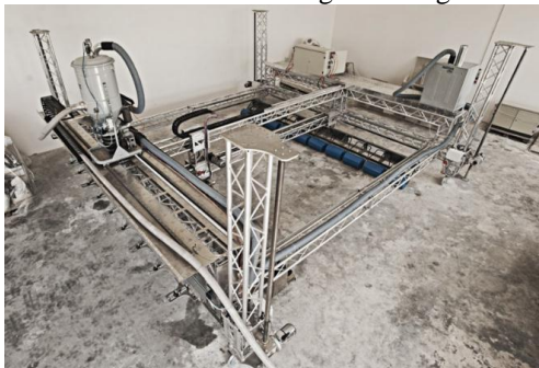
Figure 3. Gantry robot structure [11].
