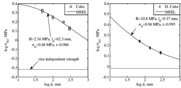
Figure 4. Modified size effect law in splitting test.
