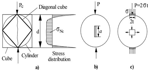
Figure 2. Splitting tension test:
