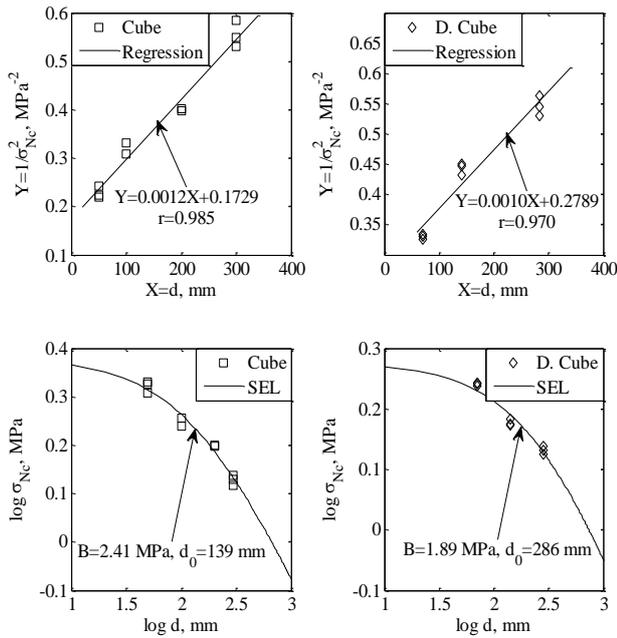
Figure 3. Size effect law in splitting test.
