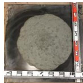
Figure 12. Slump flow (OPC-ME-MXS)
