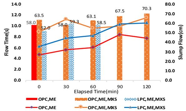
Figure 10. V funnel test results and Slump flow test results
