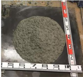
Figure 13. Slump flow (LPC-ME-MXS)
