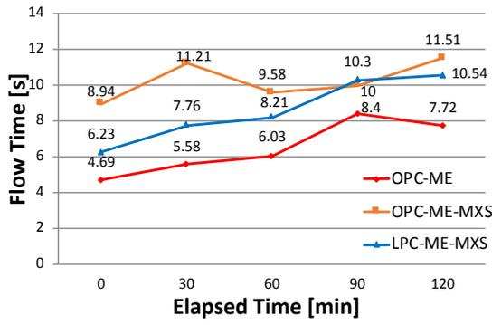
Figure 7. V funnel test results
