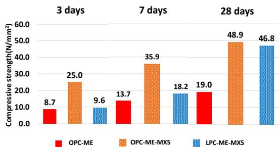
Figure 14. Compressive strength test results (Concrete)
