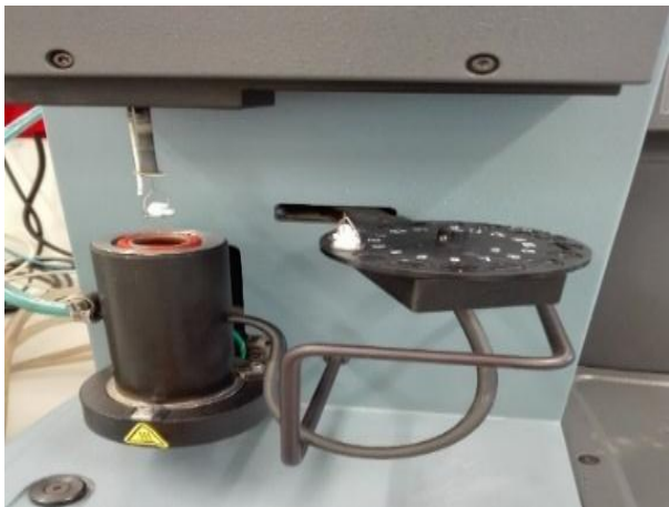
Figure 10. Samples being loaded into heat furnace
