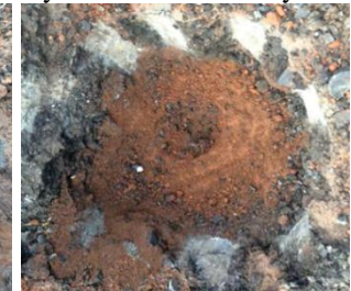
Figure 5. WBM contains moist fine particles.
