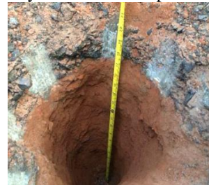
Figure 4. WBM Layer Thickness 450mm.
