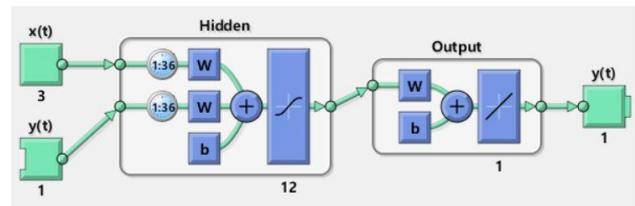
Figure 4. Matlab NARX Neural Network Series-Parallel Configuration(Training)
