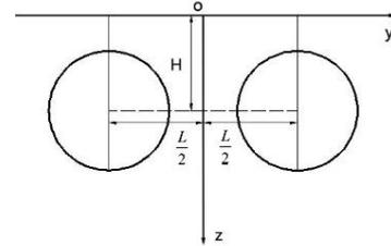
Figure 4. Calculation diagram of double-tube parallel shield tunnels
