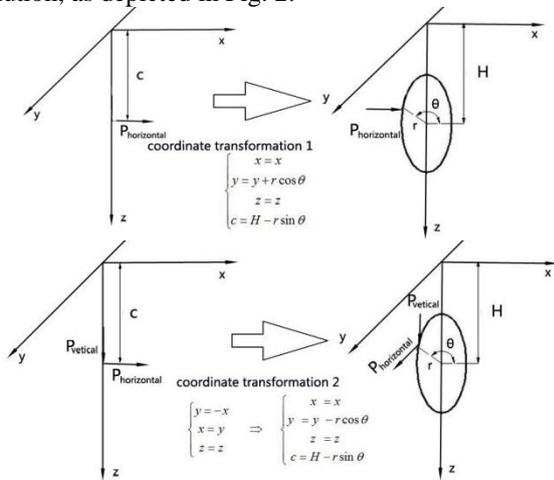
Figure 2. Calculation diagram for coordinate transformation.
