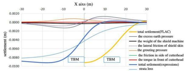
Figure 7. The result comparison of longitudinal ground settlement between expressions and numerical simulation when the left tunnel advancing 16.5 m
