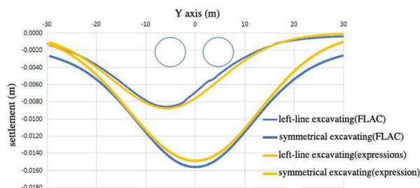
Figure 9. The result comparison of lateral ground settlement of section X=6m between expressions and numerical simulation when the double-tube tunnels advancing 22.5m.
