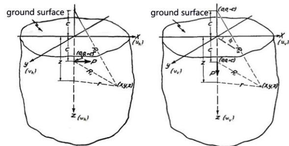
Figure 1. Force normal and parallel to the boundary in the interior of a semi-infinite solid
