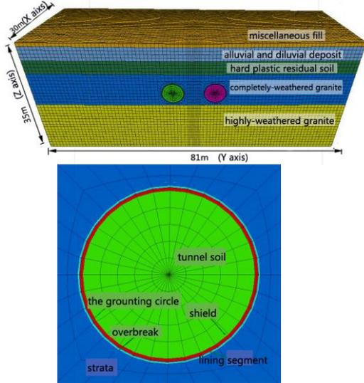
Figure 5. The classification of soil layer and the grid of surrounding rock of tunnel.
