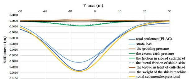
Figure 8. The result comparison of lateral ground settlement of section X=6m between expressions and numerical simulation when the left tunnel advancing 22.5 m
