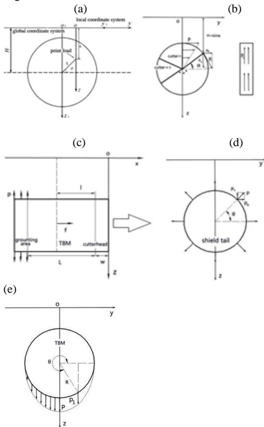
Figure 3. Calculation diagram of construction factors. (a) the excess earth pressure, (b) the lateral friction between shield skin and the surrounding soil, (c) the friction force between cutter-head and soil, (d) the grouting pressure at shield tail, (e) the gravity of the shield machine.
