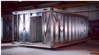
Figure 13. Typical 4-sided Load-bearing Module, courtesy – (Lawson, 2014)
