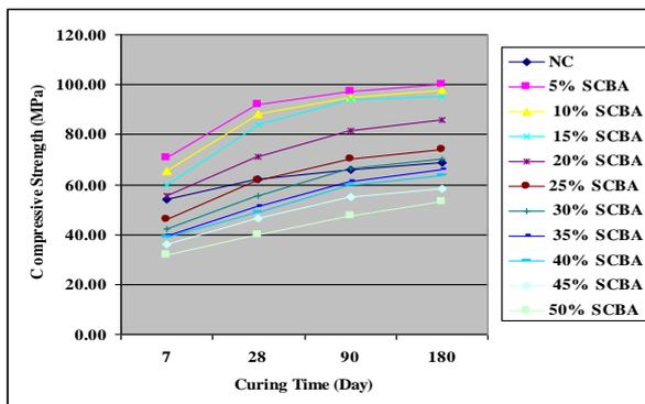
Figure 5. Effect of SCBA on the compressive strength of concrete
