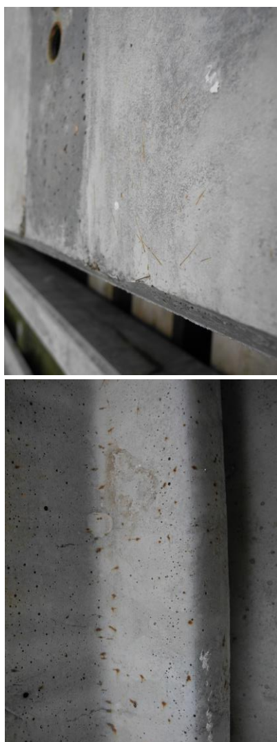
Figure 1. Surface area of UHPSFRC elements exposed to the climatic load after 1 year of exposing.
