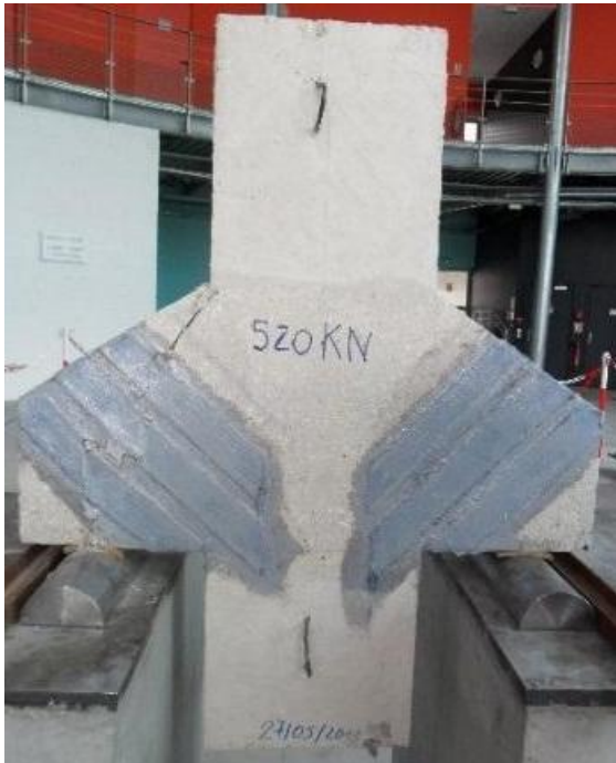
d) CI2b : Flexion and little compression failure
