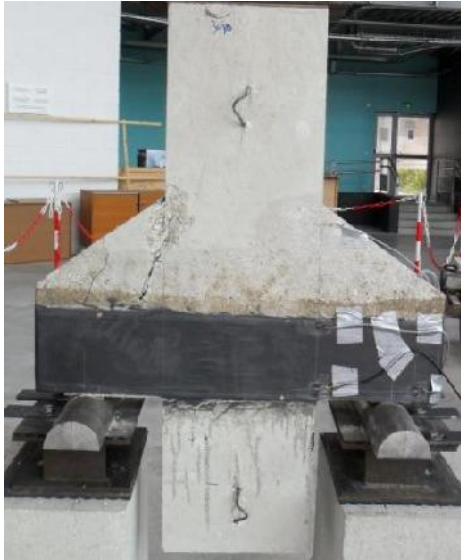
b) CB3u : Compression failure
