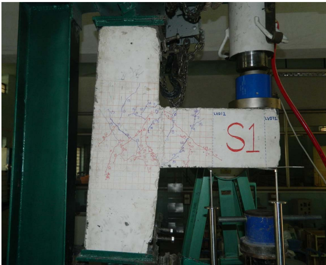
Figure 7: Crack Pattern of Joint S1
