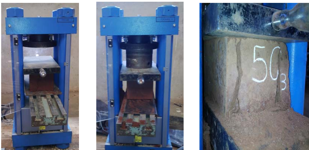
Figure 1: Compressive Strength Testing in a Universal Testing Machine
