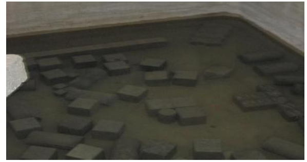
Figure 2: Curing of Concrete
