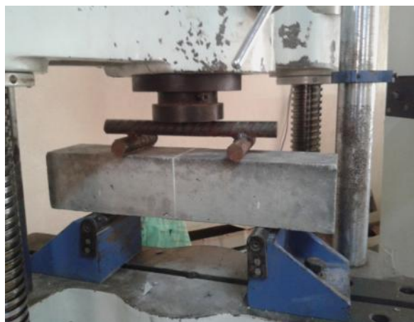
Figure 5: Flexural Test of Prism
