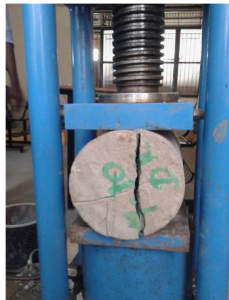
Figure 4: Split Tensile Test for Cylinder Specimen
