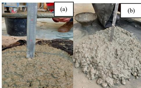
Fig. 2. Slump of specimens at different percentages of replacing aggregate by untreated CMW
