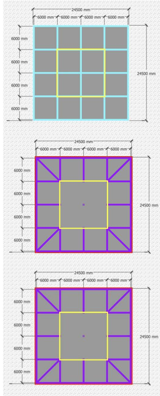
Fig. 2. Floor layout showing beam arrangement of model 1, model 2 and model 3.
