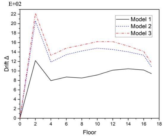
Fig. 14. Displacement in x-direction (Imperial Valley Earthquake).
