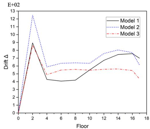
Fig. 15. Displacement in y-direction (Imperial Valley Earthquake).
