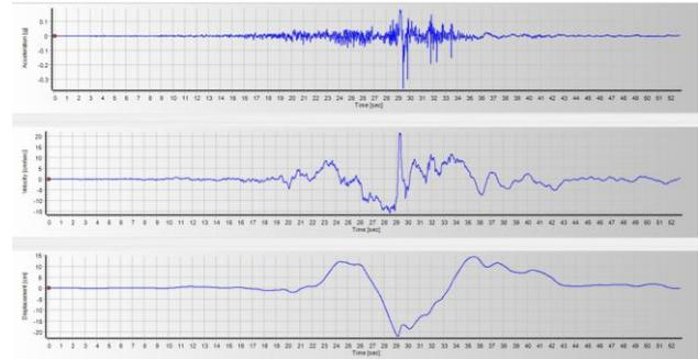
Fig. 3. Acceleration, velocity and displacement plots in the domain–Chi-Chi Earthquake.
