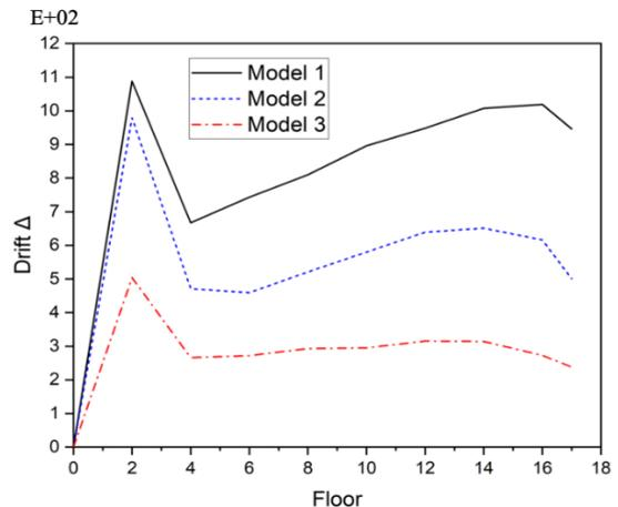
Fig. 10. Displacement in x-direction (Chi-Chi Earthquake).
