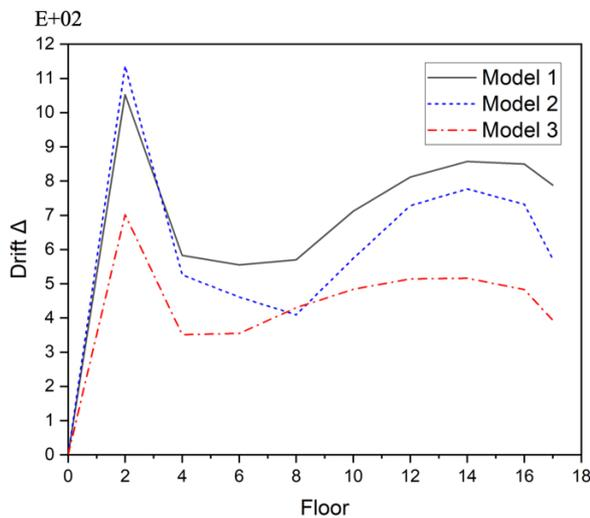
Fig. 13. Displacement in y-direction (Kobe Earthquake).
