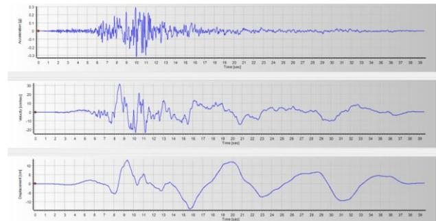
Fig. 5. Acceleration, velocity and displacement plots in the domain–Imperial Valley Earthquake.
