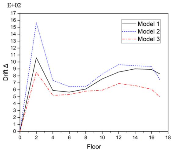
Fig. 12. Displacement in x-direction (Kobe Earthquake).
