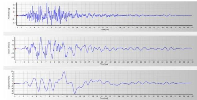
Fig. 4. Acceleration, velocity and displacement plots in the domain–Kobe Earthquake.
