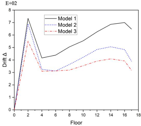
Fig. 11. Displacement in y-direction (Chi-Chi Earthquake).
