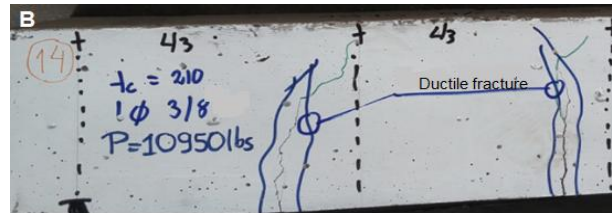
Figure 2. A) Samples of the flexural test and B) Analysis of fissures.
