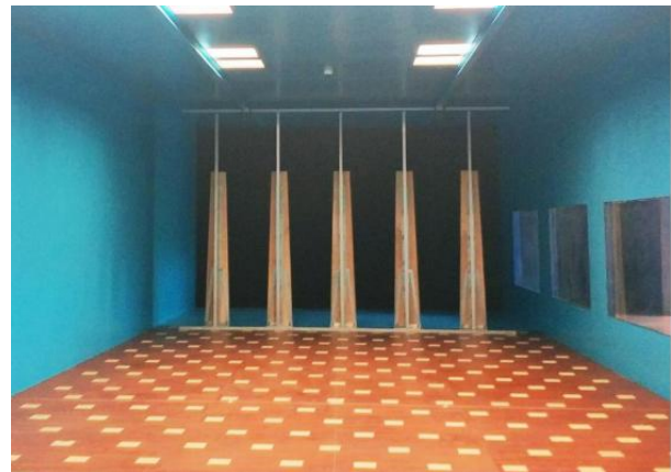
Figure 5. Wedge roughness elements in the wind tunnel lab
