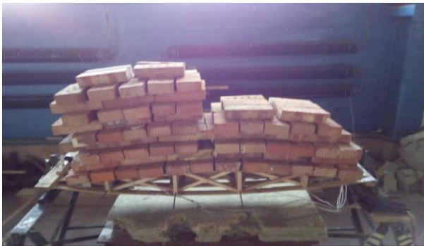
Figure 8. Loading decreased model SRS distributed one-sided load, equaled 1,5 q calculated (4,185 [kN/m 2 ] / 2,61 [kN/m 2 ]).
