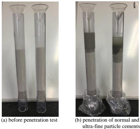
Figure 3. Column permeation tests for dry sands.
