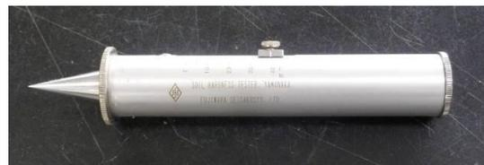
Figure 7. Portable soil hardness tester.
