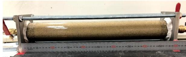
Figure 5. Column with saturated sand.
