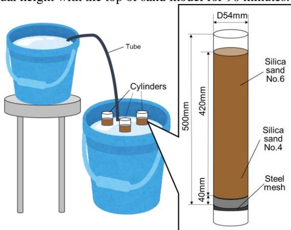
Figure 4. Saturation method of sand model.
