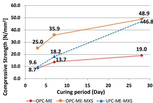
Figure 15. Compressive strength test results (Concrete)
