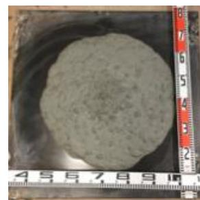
Figure 12. Slump flow (OPC-ME-MXS)
