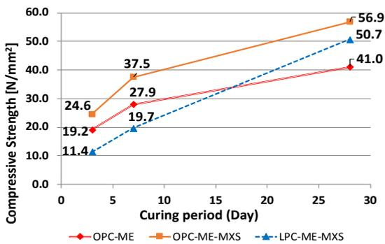
Figure 9. Compressive strength test results
