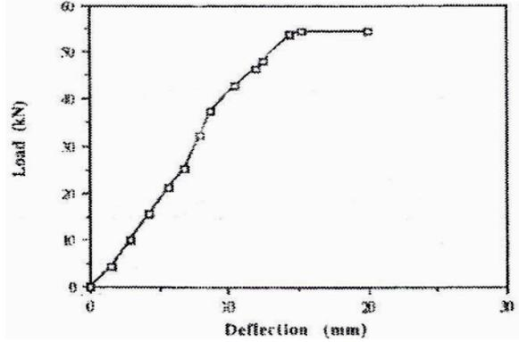
Figure 8. Beam RCONT12 showing load against deflection.
