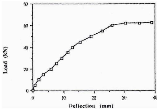
Figure 6. Beam RCON3 showing load against deflection.
