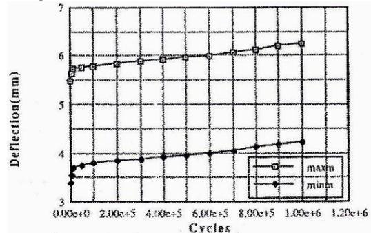
Figure 3. Beam RCON3 First Cycled at Service Loading to 1M cycles, before being Tested Statically.
