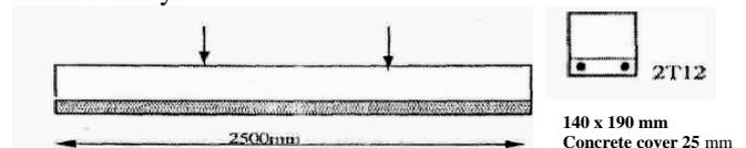
Figure 1. Beam and fault dimensions, shear force & bending moment diagrams.
