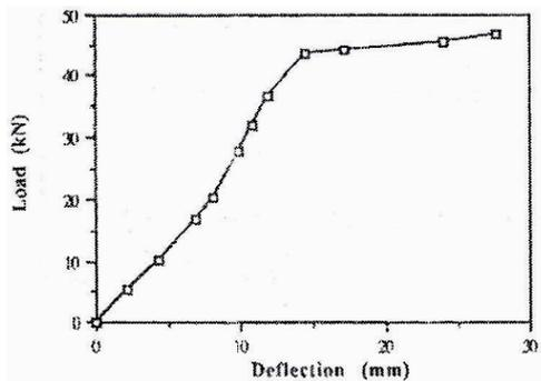
Figure 7. Beam RCEM6 showing load against deflection.
