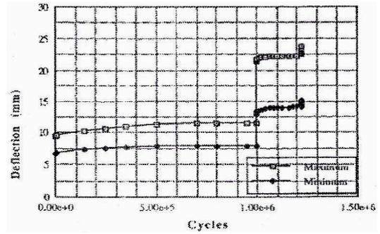
Figure 13. Beam RCONT10, first cycled at service loading to 1M cycles, then to failure at near ultimate.
