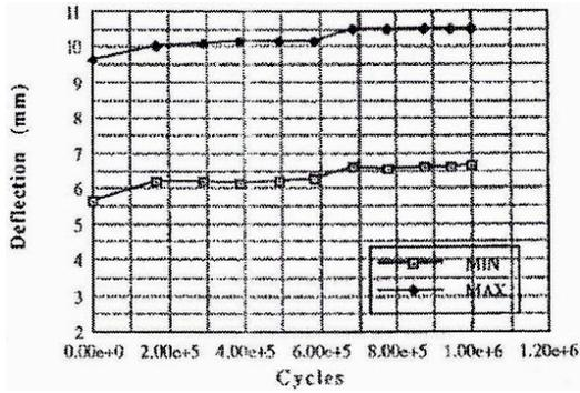
Figure 4. Beam RCEM6 first cycled at service loading to 1M cycles, before being tested statically.
