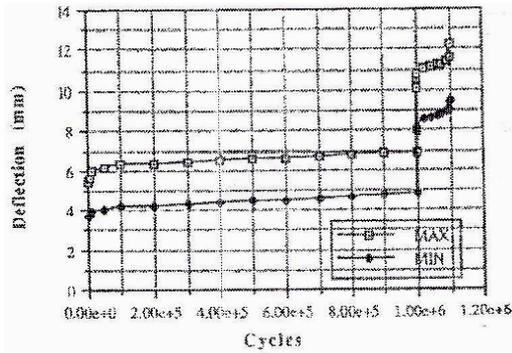
Figure 10. Beam RCON2 First Cycled at Service Loading to 1M cycles, then to failure at Near Ultimate.
