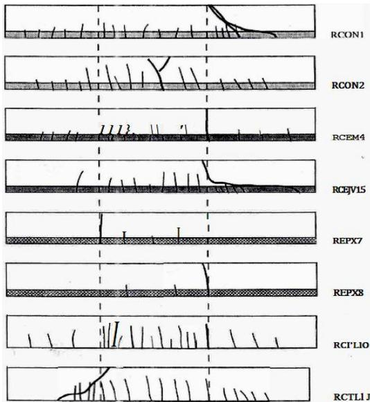
Figure 2. Crack pattern of tested beams.
