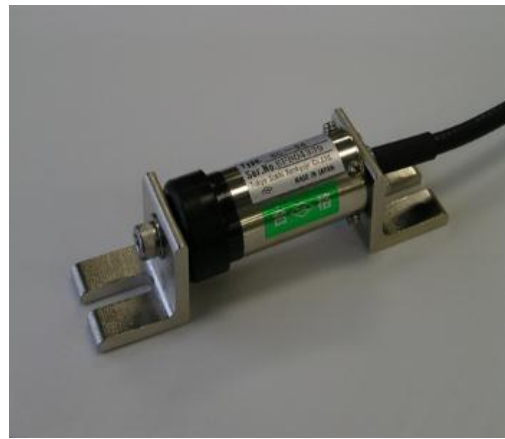
Figure 6. Crack Width meter
