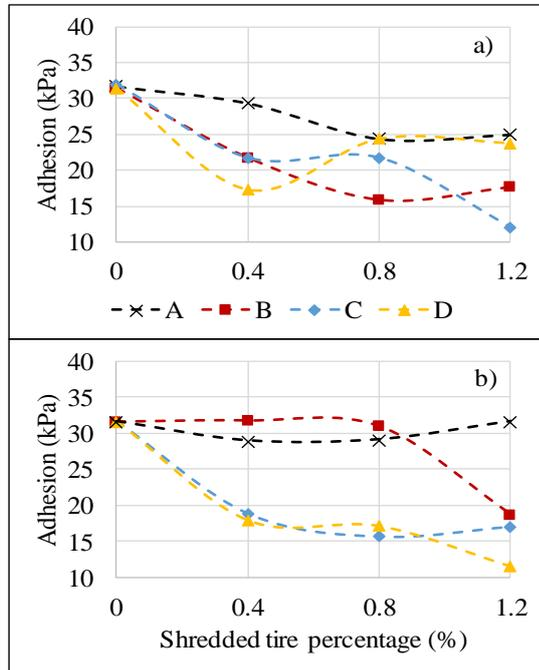
Figure 6. Adhesion of unreinforced and reinforced soil samples versus the percentage of shredded tire with different dimensions: a) shredded tire sheet; b) shredded tire fiber.
