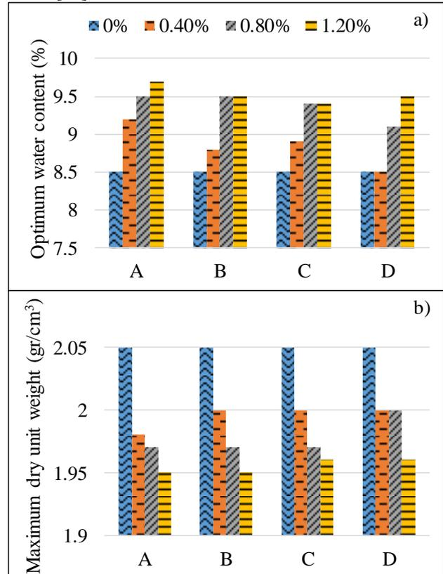
Figure 2. a) Maximum dry unit weight variation of unreinforced and reinforced soil samples with different percentages and sizes of fiber shredded tire; b) optimum water content variation of unreinforced and reinforced soil samples with different percentages and sizes of fiber shredded tire
