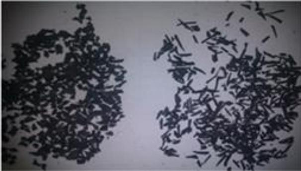
Figure 1. Two types of sheet and fiber shredded tires
