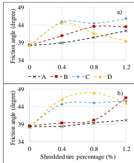
Figure 5. The friction angle of unreinforced and reinforced soil samples versus the percentage of shredded tire with different dimensions: a) shredded tire sheet; b) shredded tire fiber.
