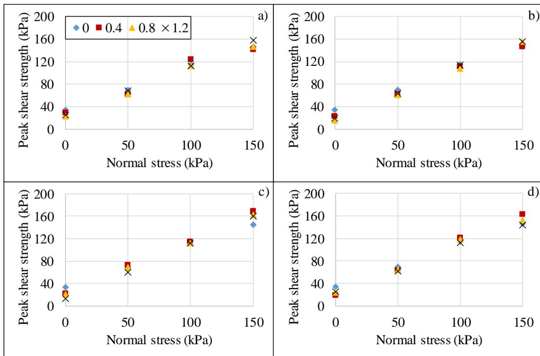
Figure 3. The peak shear strength versus normal stress of unreinforced and reinforced soil samples with shredded sheet tire with dimensions: a) A; b) B; c) C; and d) D.
