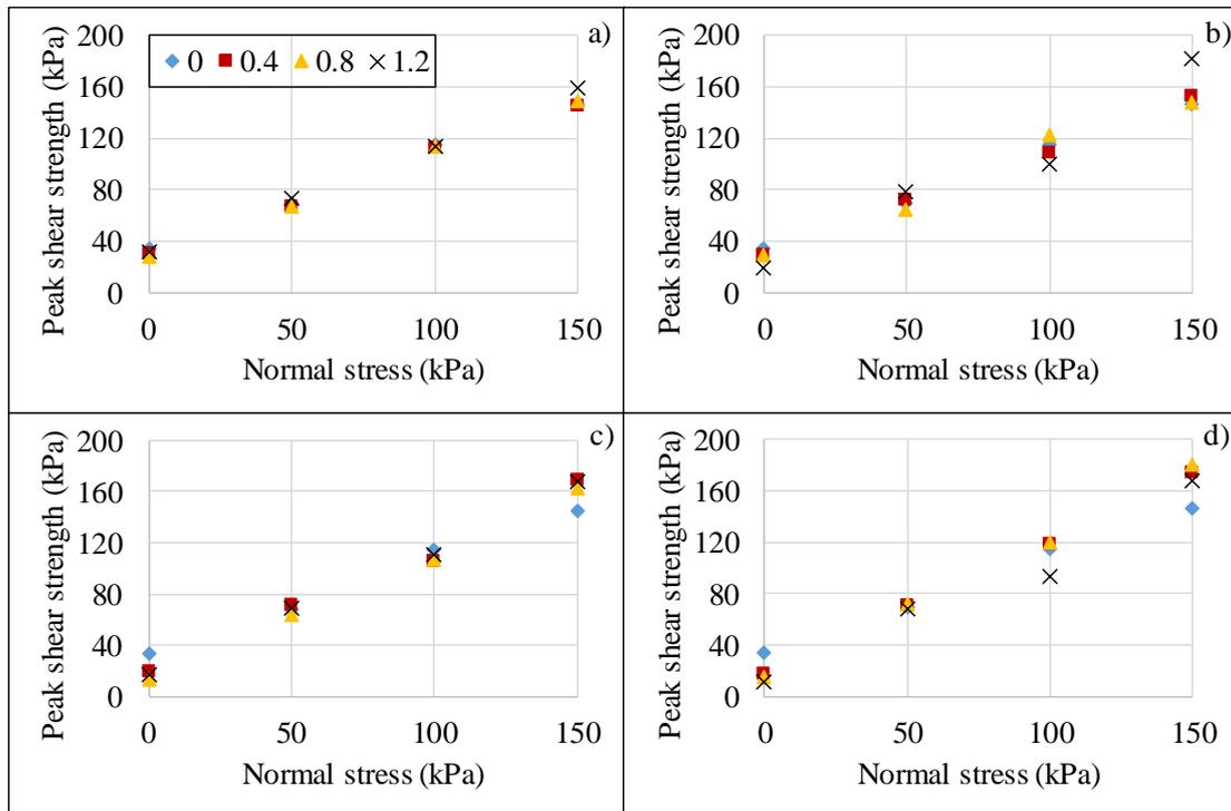
Figure 4. The peak shear strength versus normal stress of unreinforced and reinforced soil samples with shredded fiber tire with dimensions: a) A; b) B; c) C; and d) D
