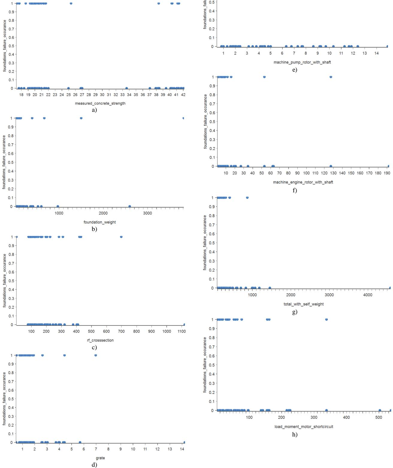
Figure 2. The scatter plots – target versus input variables: a) Measured concrete strength [MPa], b) The weight of the foundation [kN], c) Cross-section reinforcement [cm<sup>2</sup>], d) Grate [kN], e) The pump unit and rotor with shaft [kN], f) The engine unit and rotor with shaft [kN], g) Total load with fund. self-weight [kN], h) Load from motor short circuit [kNm]. Target variable is the foundation failure occurrence [1- yes, 0 -no]
