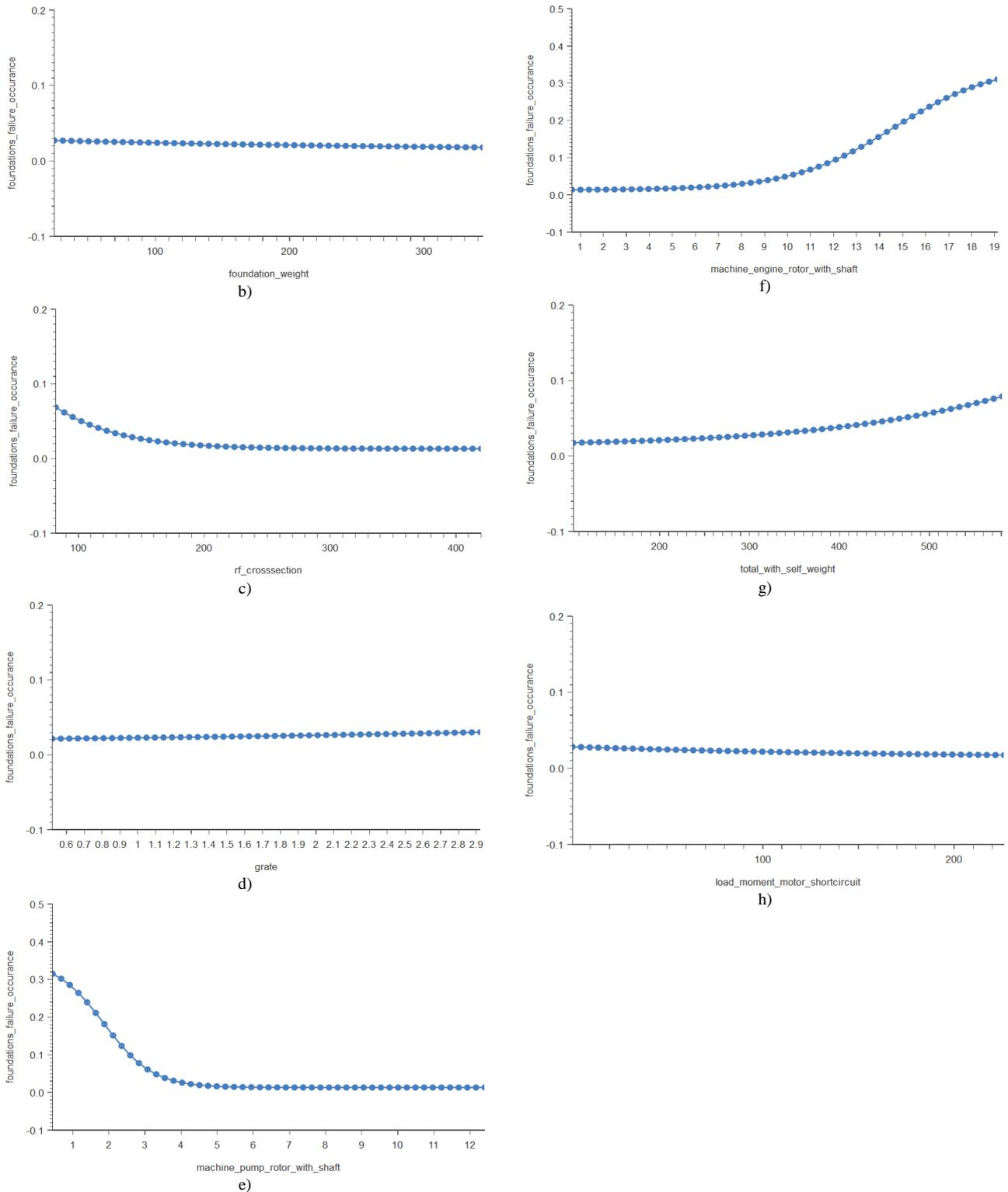
Figure 7. Output charts - the diagrams show fluctuations in output variables for a single input variable, while the others are fixed: a) Measured concrete strength [MPa], b) The weight of the foundation [kN], c) Cross-section reinforcement [cm<sup>2</sup>], d) Grate [kN], e) The pump unit and rotor with shaft [kN], f) The engine unit and rotor with shaft [kN], g) Total load with fund. self-weight [kN], h) Load from motor short circuit [kNm]. Target variable is the foundation failure occurrence.
