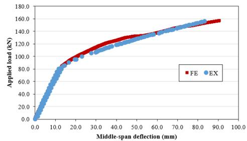
Figure 6. Relationships between applied load and middle-span deflection.
