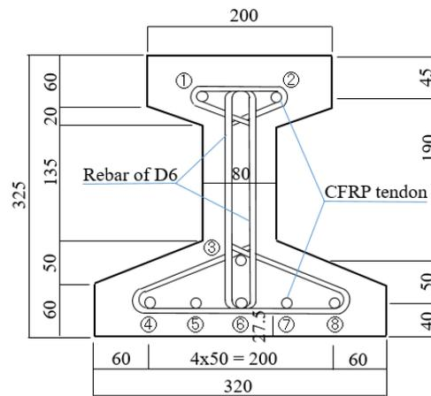
Figure 3. Cross-section of Shinmiya Bridge (unit: mm)
