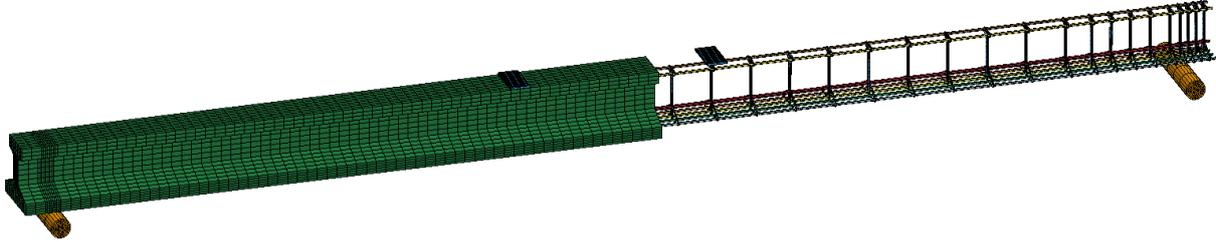
Figure 5. Three-dimensional analysis model for experiment girder
