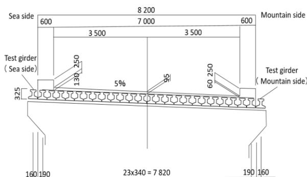
Figure 2. Cross-section of Shinmiya Bridge (unit: mm)
