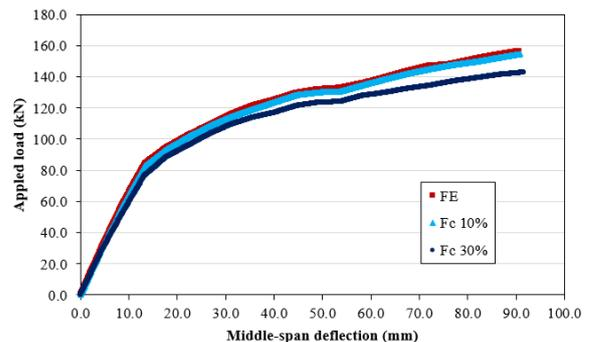
Figure 9. Relationships between applied load and middle-span deflection corresponding to the difference value of compressive strength of concrete
