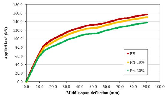
Figure 8. Relationships between applied load and middle-span deflection corresponding to the level of pre-stressing force.
