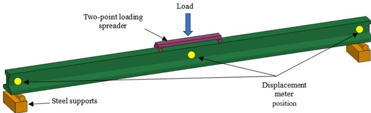
Figure 4. Setup of the experiment for Shinmiya bridge girder
