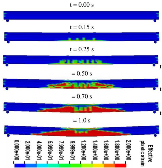
Figure 7. Deformation and strain situation in several stages of simulation.
