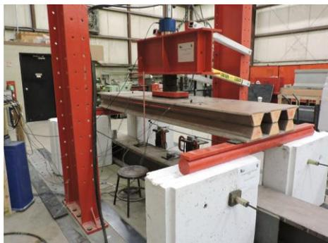
Figure 2. Static flexural test setup
