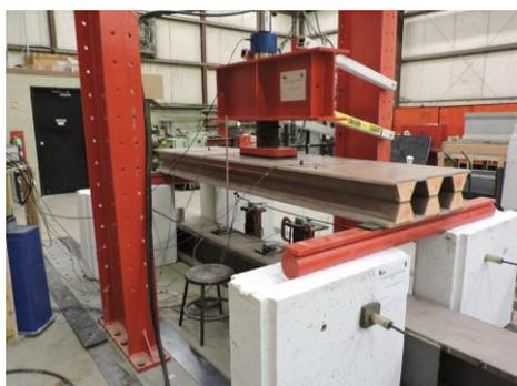
Figure 2. Static flexural test setup
