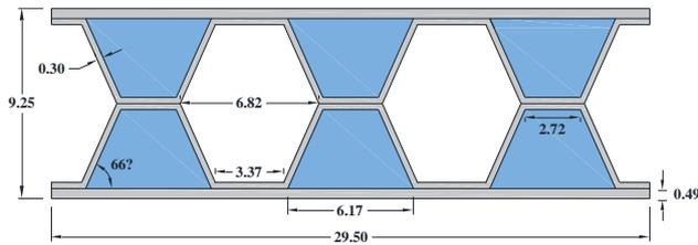
Figure 1. Overall sandwich panel bridge deck, all dimensions in inches (1 in. = 25.4 mm)
