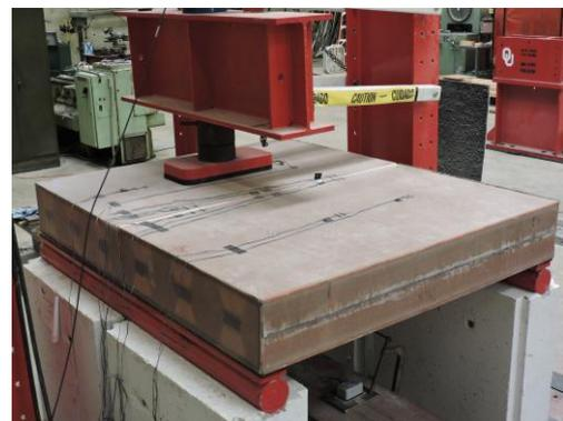
Figure 4. Static flexural test setup for panel-to-panel joint connect
