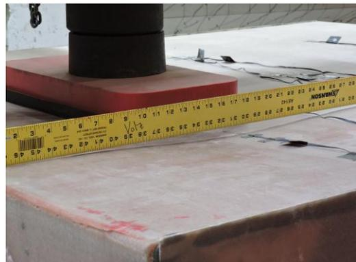
Figure 8. Bearing Failure underneath the point load
