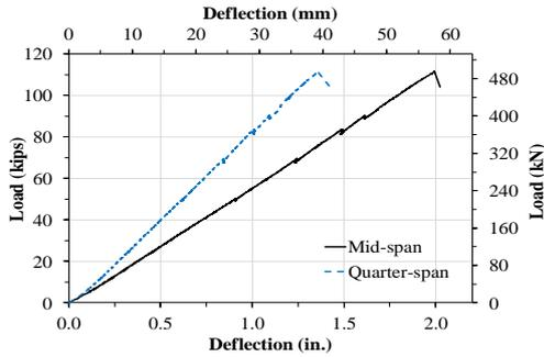
Figure 5. Load-deflection curve at mid-span and quarter-span of the panel
