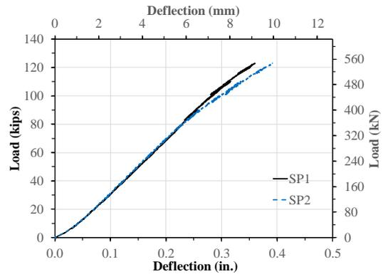
Figure 7. Load-deflection curves at each panel edge adjacent to the bonded joint
