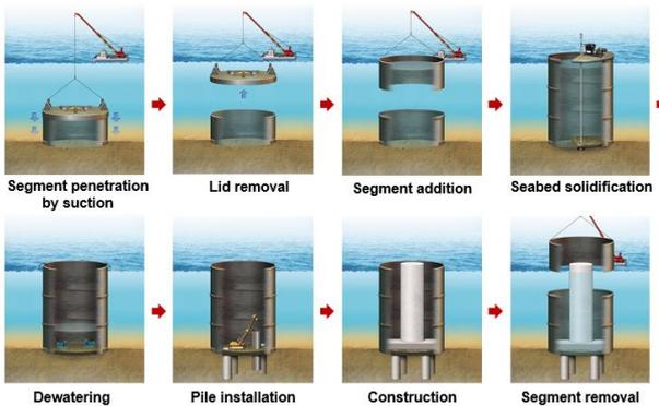
Figure 1. Construction procedure of offshore single large cofferdam
