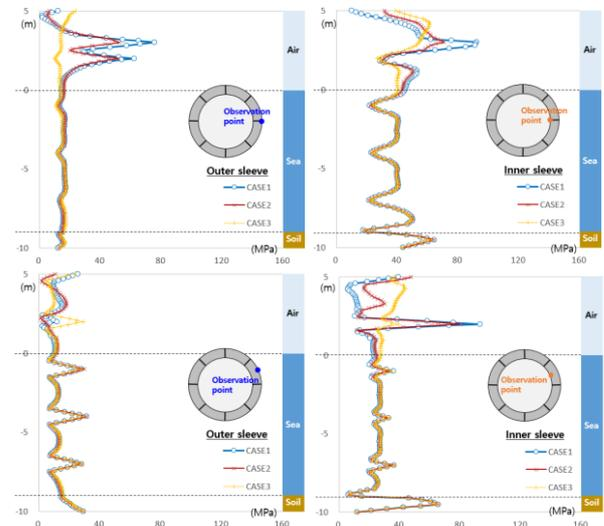
Figure 6. Stress profiles (bottom segment, initial penetration)
