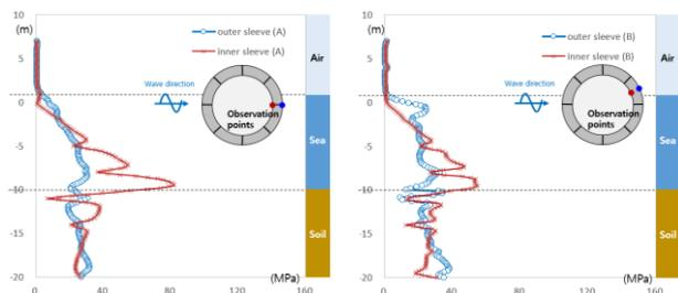
Figure 10. Stress profiles (dewatering, rear)
