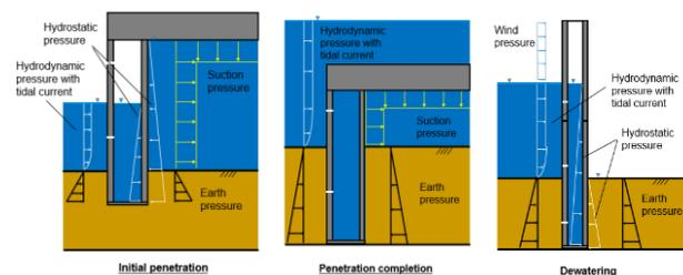
Figure 3. Applied load diagrams
