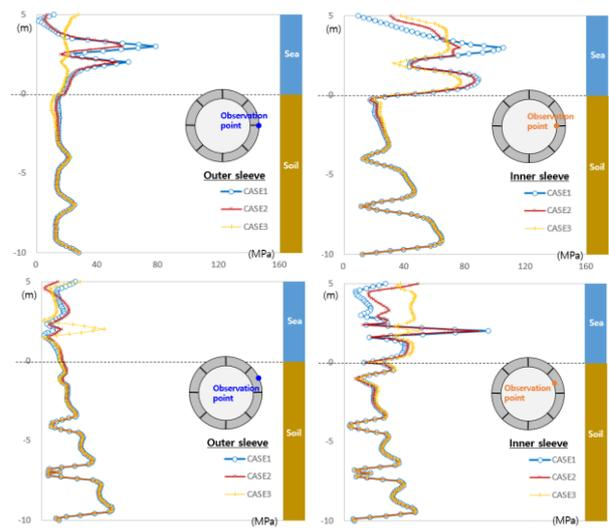
Figure 7. Stress profiles (bottom segment, penetration completion)
