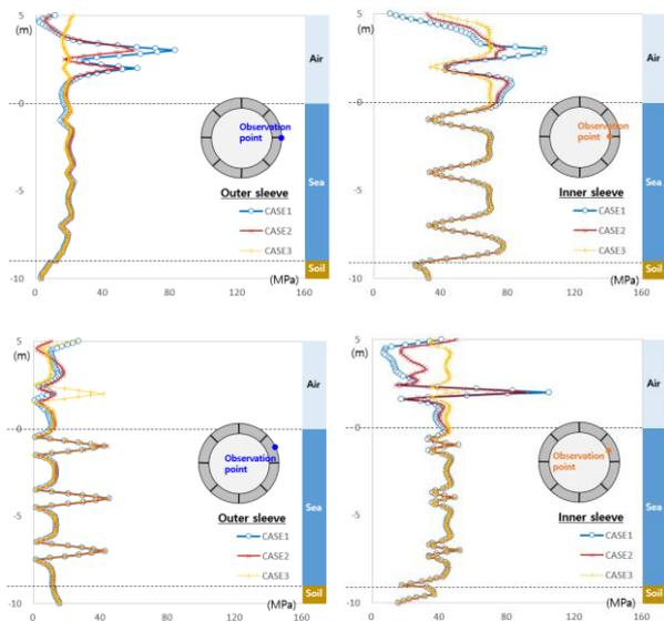
Figure 5. Stress profiles (bottom segment, only confinement loadings)
