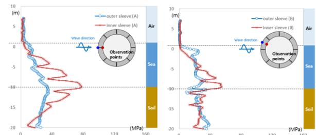
Figure 8. Stress profiles (dewatering, front)
