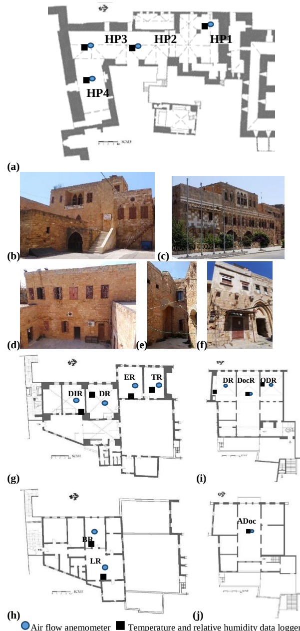
Figure 1. Case study sites and the equipment locations: (a) The plan of the public multifunctional gallery (G), (b) Eastern facade of the Technical Office (T), (c) The western facade of the Technical Office (T), (d) The northern facade of Department of Antiquities (D), (e) The Department of Antiquities (D) from the alley, (f) The Print shop (g) Ground floor plan of (D) (h) First-floor plan of (D) (i) Ground floor plan of (T) (j) First-floor plan of (T)
