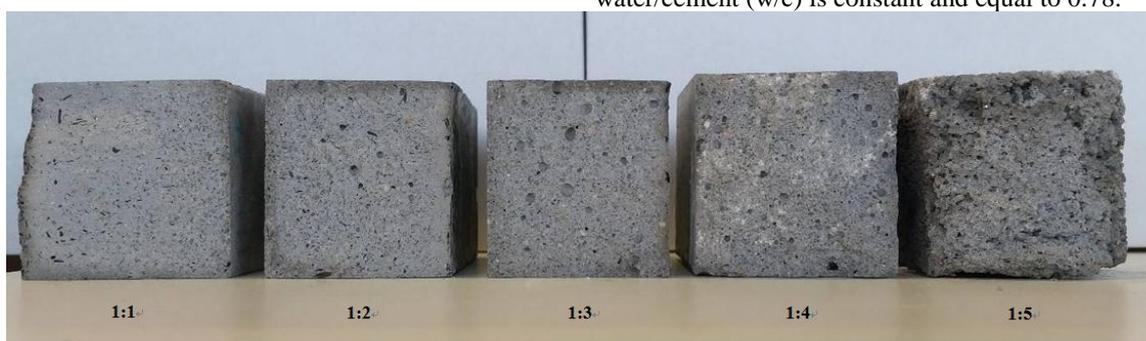
Figure 1. Novel GP-mortars cross sections showing an increasing porosity in relation to aggregates amount.
