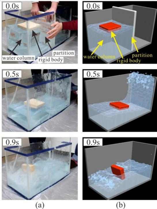
Figure 4. Dam break problem (a) experimental results (b) numerical results.
