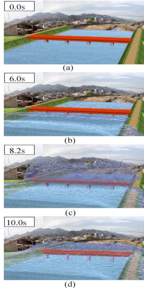
Figure 7. Numerical results for 3-D washout analysis of the bridge superstructure.
