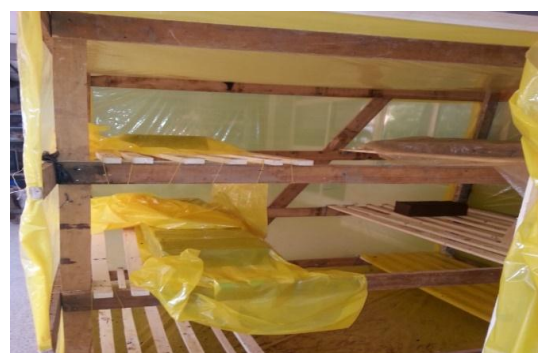
Figure 2. Plastic curing shelter.
