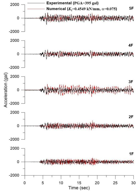
Figure 6. Comparison of the experimental and numerical seismic acceleration responses obtained from nonlinear time history analysis (PGA=395 gal).
