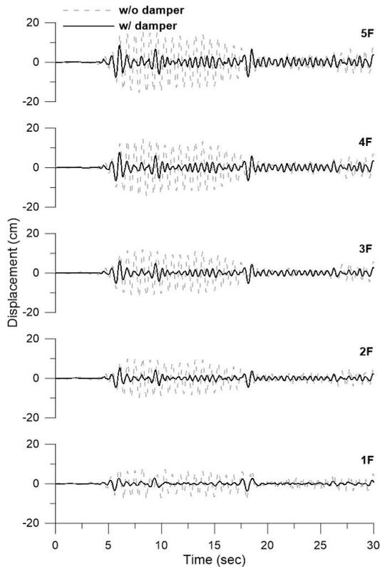
Figure 5. Comparison of the seismic displacement responses with and without the in-plane arch-shaped dampers (PGA=395 gal).
