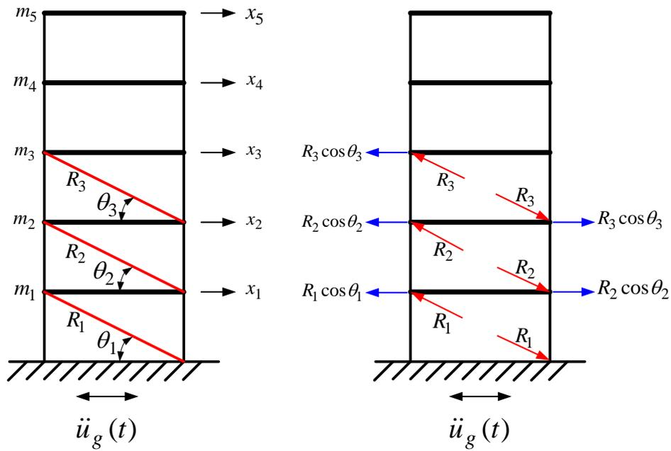
Figure 2. The restoring forces of the in-plane arch-shaped dampers considered in the nonlinear time history analysis of the 5-story steel model frame.
