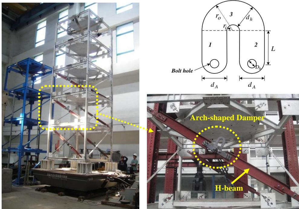
Figure 3. Experimental setup of a 5-story steel model frame implemented with in-plane arch-shaped dampers.
