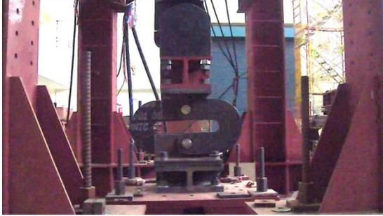
Figure 1. In-plane arch-shaped damper [23].
