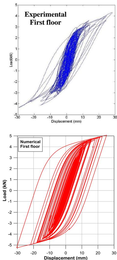
Figure 8. Simulated hysteresis loops of the in-plane arch-shaped dampers implemented on the first story of the 5-story steel model frame (El Centro earthquake, PGA=395 gal).
