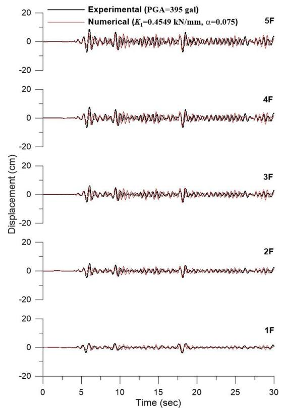
Figure 7. Comparison of the experimental and numerical seismic displacement responses obtained from nonlinear time history analysis (PGA=395 gal).
