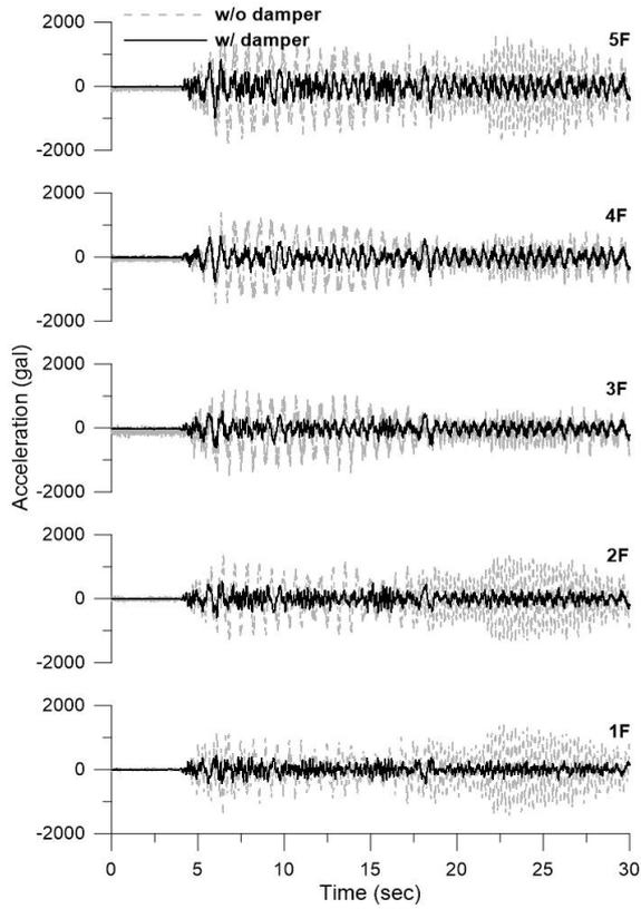
Figure 4. Comparison of the seismic acceleration responses with and without the in-plane arch-shaped dampers (PGA=395 gal).
