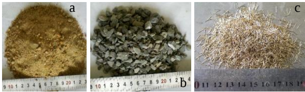
Figure 1. apparent shape of (a) river sand, (b) crushed stone, (c) steel fiber.
