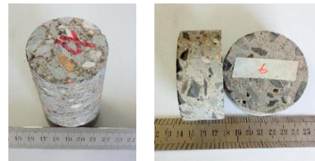
Figure 3. Typical test specimen: (a) Uniaxial compression test, (b) Brazilian disc splitting and SHPB test.
