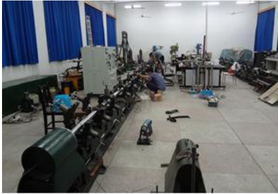
Figure 5. The device of large diameter split Hopkinson pressure bar
