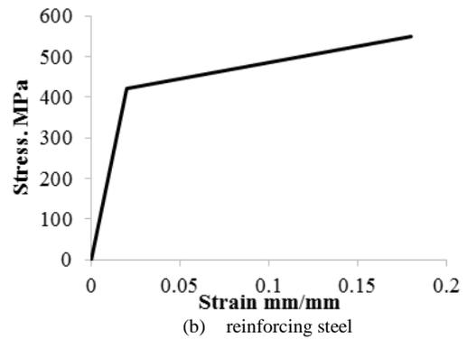
Figure 2. Stress-strain curves.
