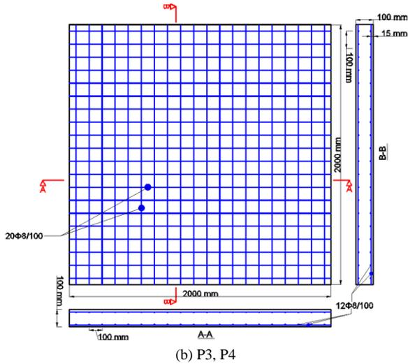
Figure 1. Reinforcement plan for typical RC plates.
