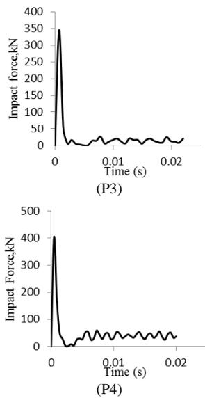
Figure 3. Impact force-time curves of RC plates(kN-s).
