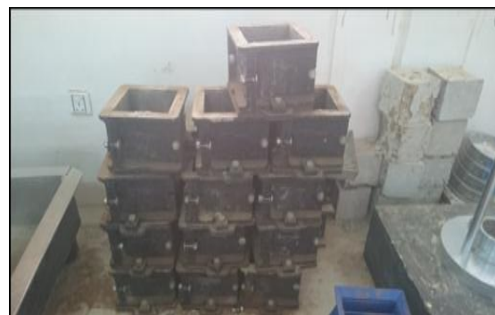
Figure 2. Cubes USING IN CASTING CONCRETE
