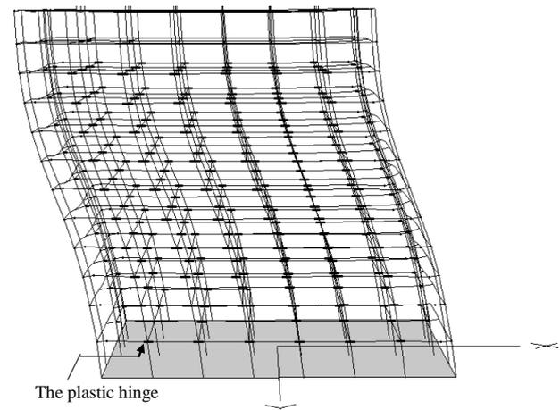
Figure 7. The maximum deformation state of the reference building. (JMA-Kobe, 50 kine)
