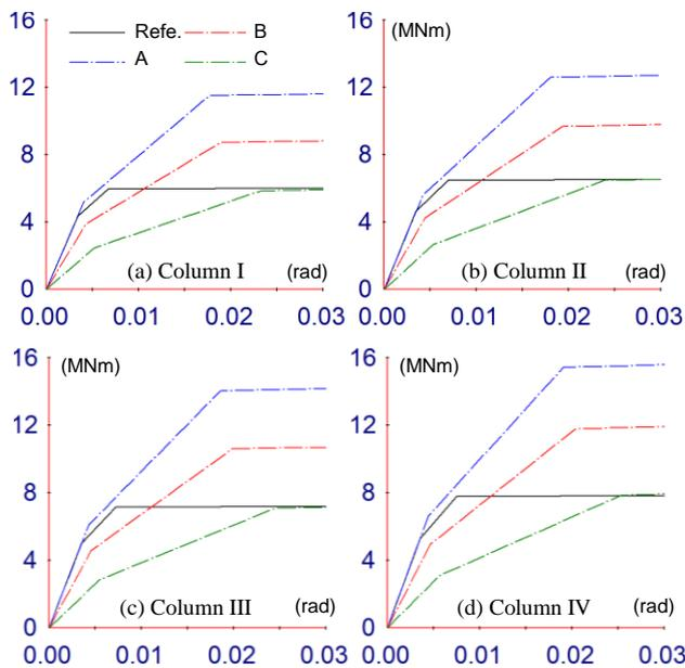
Figure 5. Result of static incremental analysis of each models.
