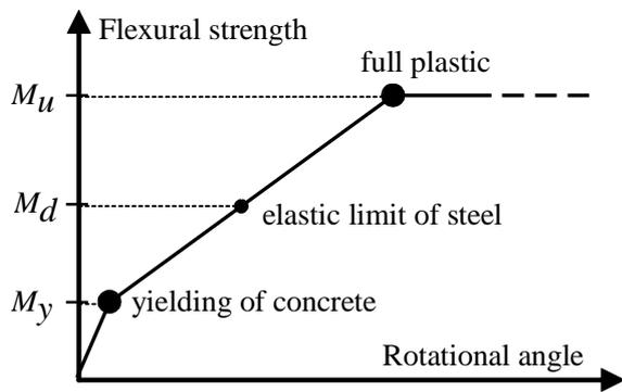
Figure 3. Flexural strength - rotational angle relationship of the CFT column member [8].
