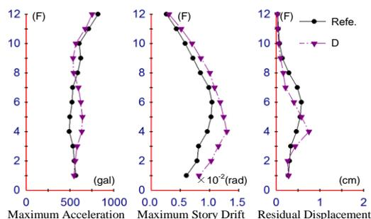
Figure 11. Dynamic analysis result of Model D. (JMA-Kobe NS 75kine)
