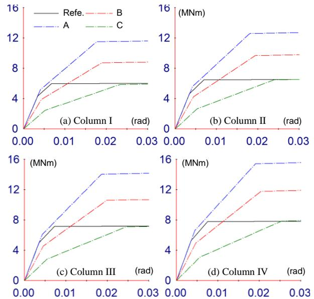
Figure 4. The flexural strength - rotational angle relationship of each CFT columns.
