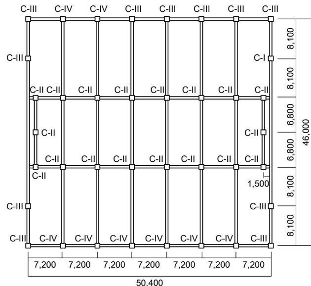
Figure 1. The ground floor plan of target building. (Unit: mm)
