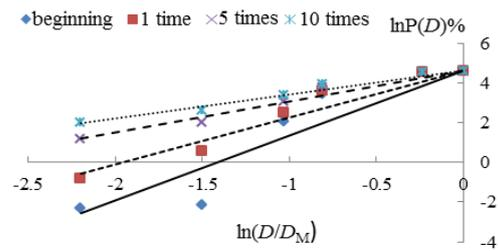
Figure 5. The degree of basalt particles breakage under cycle loading
