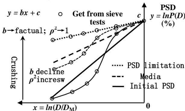
Figure 1. The revolution of fitting line of particle grading contributed by particle crushing
