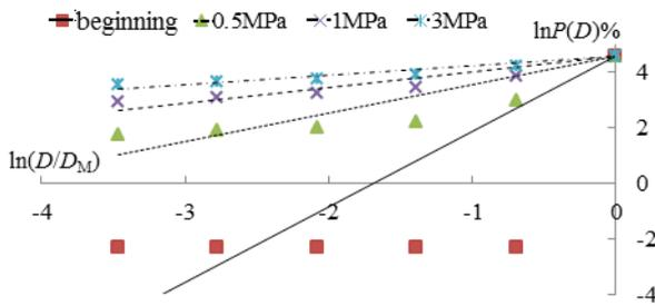
Figure 4. Evolution of grain-size distribution after monotonic loading of Mayoraz
