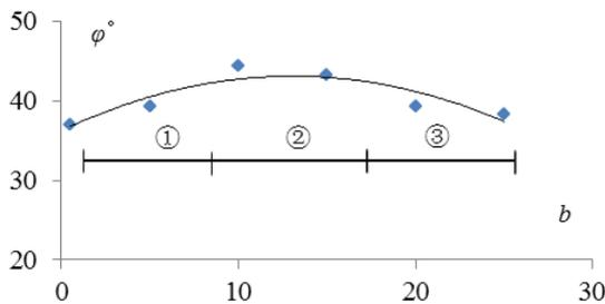
Figure 8. The relationship between the parameters of particle crushing state  $b$  and strength index  $\phi$
