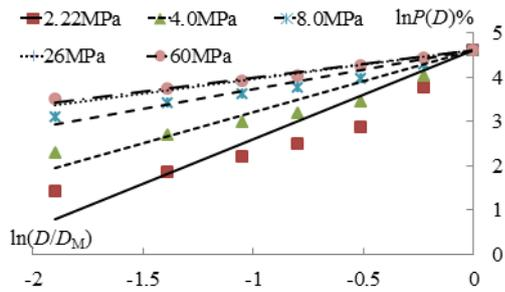
Figure 3. Evolution of grain-size distribution curves for drained triaxial compression tests of Lade
