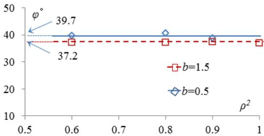
Figure 7. The relationship between the parameters of particle crushing state  $\rho^2$  and strength index  $\phi$
