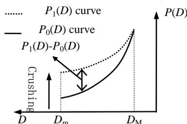
Figure 2. The sketch map of the revolution of grading with particle crushing
