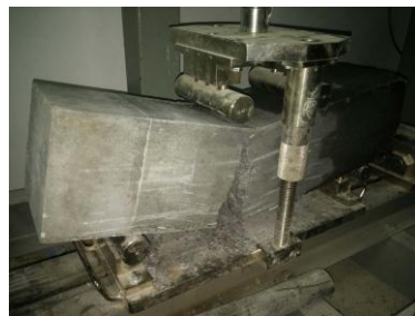
Figure 5. Examinations the type "3" Mix Design -behavior of sample-1% SF
