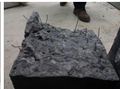
Figure 5. Examinations the type "3" Mix Design -behavior of sample-1% SF
