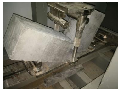
Figure 4. Examinations the type "1" Mix Design - behavior of sample-plain concrete
