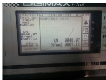
Figure 6. Examinations the type "5" Mix Design -behavior of sample-0.05% PPF
