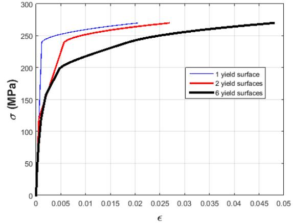
Figure 4. The stress-strain behaviors for cases when number of yield surface  $N = 1, 2$  and  $6$ .
