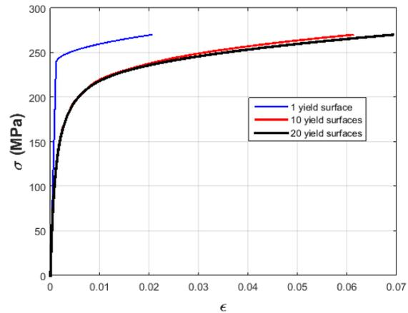
Figure 5. The stress-strain behaviors for cases when number of yield surface  $N=1, 10$  and  $20$ .
