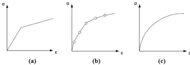
Figure 3. The stress-strain responses in cases of a) bilinear, b) piecewise linear and c) nonlinear
