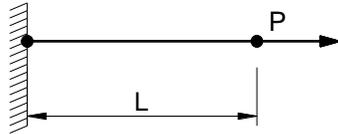
Figure 2. 1-D Finite element model.
