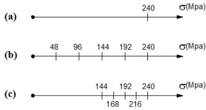
Figure 6. Distribution of yield strength of yield surfaces in case of a) 1 yield surface, b) 5 yield surfaces and  $\eta_0^{initial} = 0$  and c) 5 yield surfaces and  $\eta_0^{initial} = 0.5$
