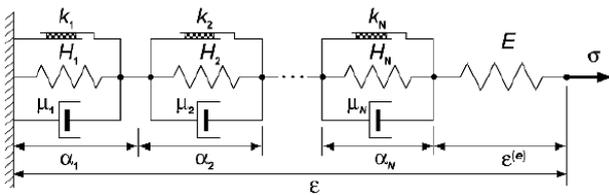
Figure 1. Mechanical behavior of multiple-yield-surface model.
