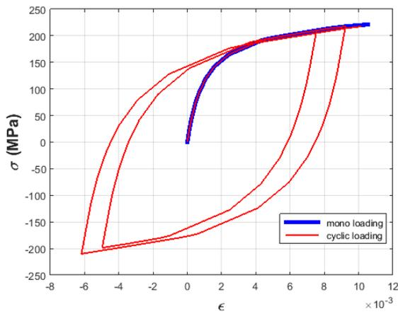
Figure 10. Behaviors of multiple-yield-surface model under mono loading and cyclic loading.
