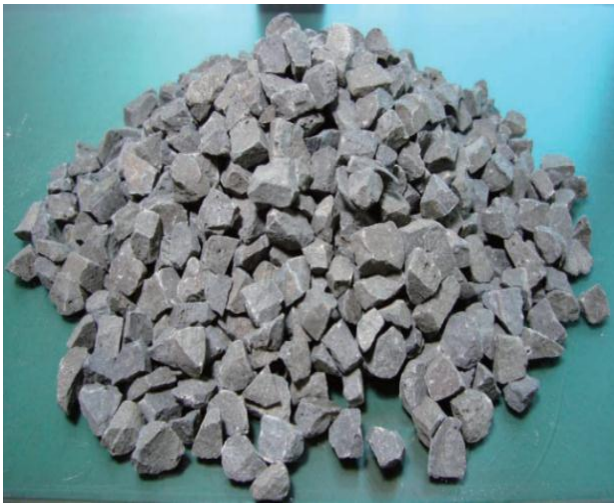
Figure 1. Physical Appearance of Reduced Air-cooled Slag Aggregate (PACSS's aggregate)
