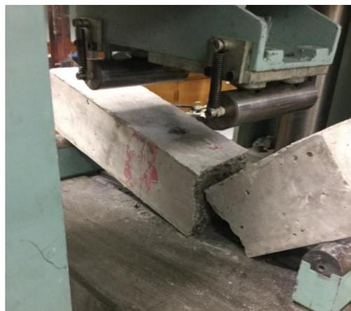
Figure 5. Typical test beams fracture under the vertical load
