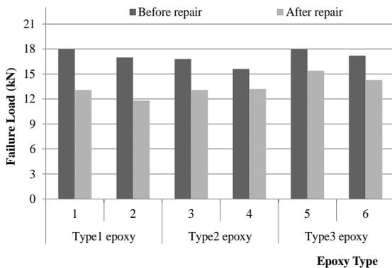
Figure 8. Flexural test results (maximum failure loads) for tested beams
