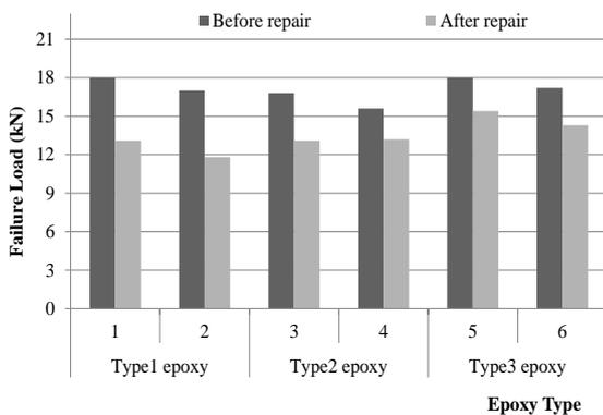
Figure 8. Flexural test results (maximum failure loads) for tested beams
