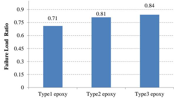
Figure 9. Average failure load ratios for beams repaired using the three epoxy products.
