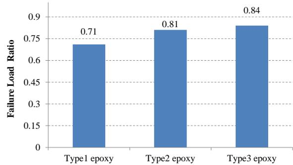
Figure 9. Average failure load ratios for beams repaired using the three epoxy products.
