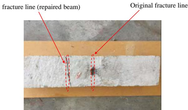
Figure 7. Failure away from the original fracture line (away from the epoxied sections) - Typical scenario for beams repaired by Type2 and Type3 epoxies
