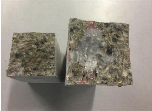
Figure 6. Failure through the epoxied section (original fracture line) – Typical scenario for beams repaired by Type1 epoxy
