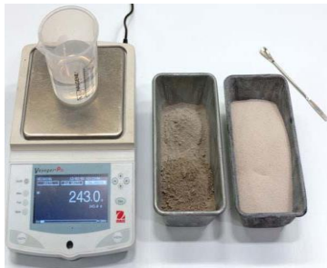
Figure 1. The demonstration of dried bulk density measurement
