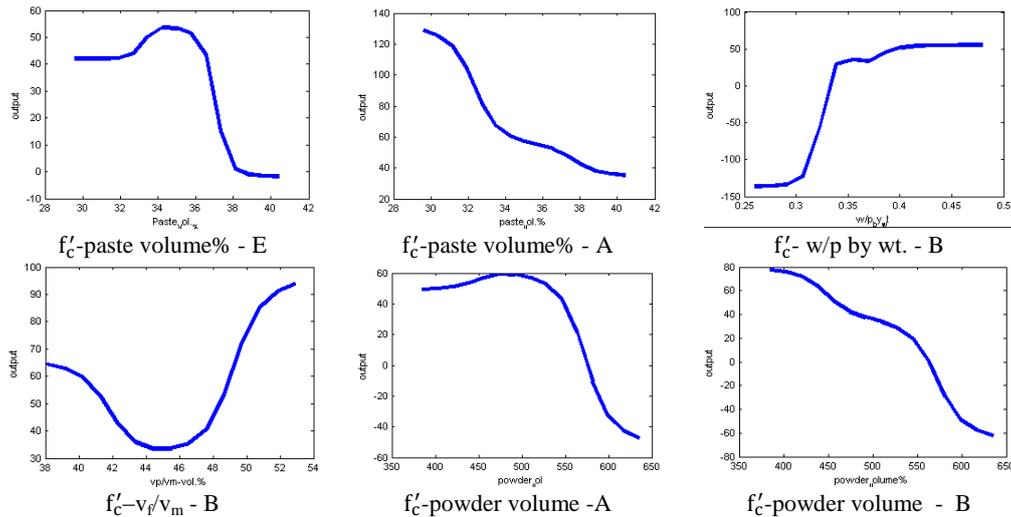
Figure 6. Particular neuro-fuzzy relationship of mixture proportion and slump flow with the compressive strength
