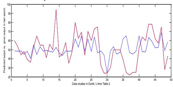
Figure 4. Predicted vs. real compressive strength at the last epoch in combinations A, B.
