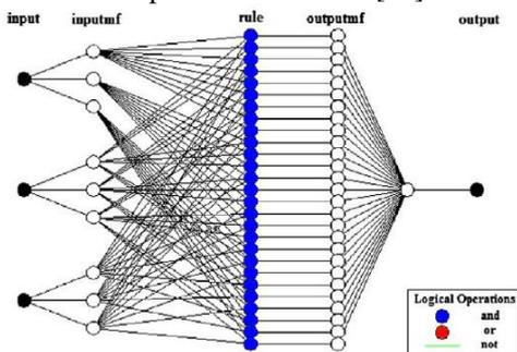
Figure 1. The structure of ANFIS network
