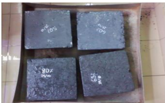
Figure 3. Specimens for big shear box after 28 days curing
