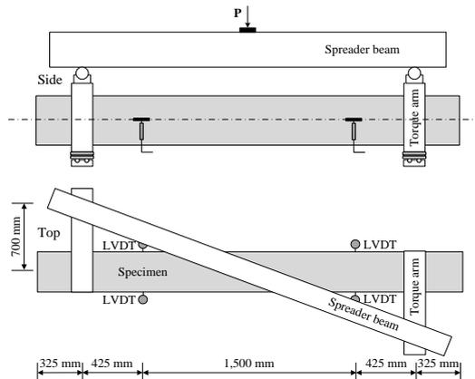
Figure 4. Loading condition and location of LVDTs.
