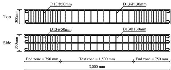
Figure 2. Configuration of the test specimens.
