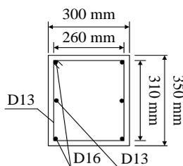
Figure 1. Section of the specimens.
