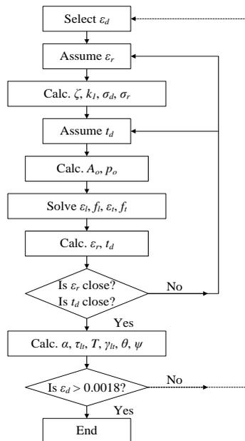
Figure 6. Flow chart of CATM for torsion.
