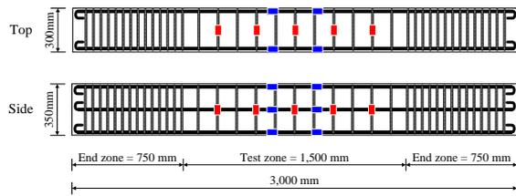
Figure 3. Location of strain gauges.
