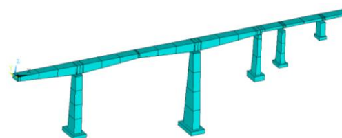
Figure 2. Three dimensional finite element model of bridge
