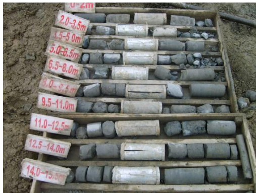
Figure 3. Drilled cores from restraint reinforced cement-soil pile.
